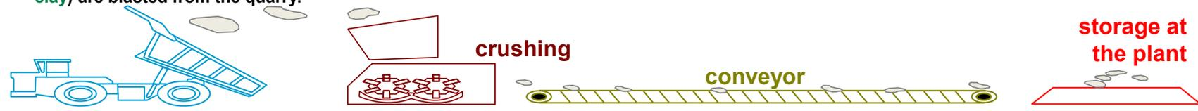
**3. CRUSHING & TRANSPORTATION:** The raw materials, after crushing, are transported to the plant by conveyor. The plant stores the materials before they are homogenized.
